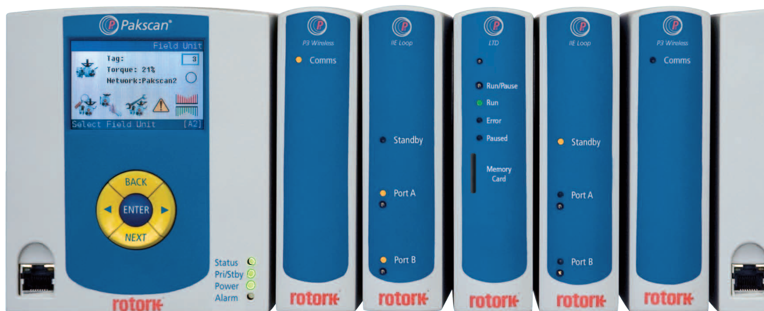
The Pakscan P3 master station with wireless capability is the bridge between the facility's host control system and the Pakscan wireless coordinator. Communication between the host and Pakscan P3 master station uses industry-standard Modbus protocol.
