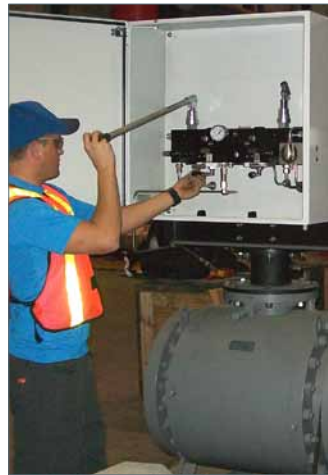
An engineer at the C E Franklin workshop tests the hydraulic manual override on one of the Rotork gas-over-oil actuators (model number GO-085S-180H/D1) bound for the Tupper West Gathering System.
