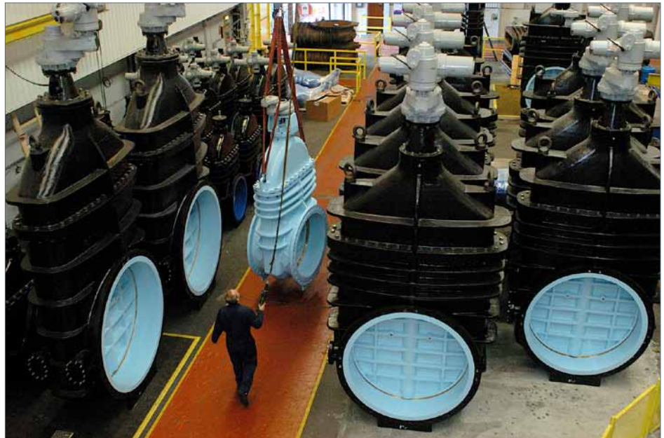
Rotork IQ Pro actuators fitted to gate valves in sizes up to DIN 1800, destined for the Doha North Sewage Treatment Works. (Photograph by kind permission from Glenfield Valves Ltd).
