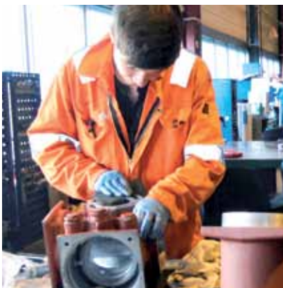
The workshop in Norway, busy motorising valves with IQ actuators for the Oseberg offshore platform project
