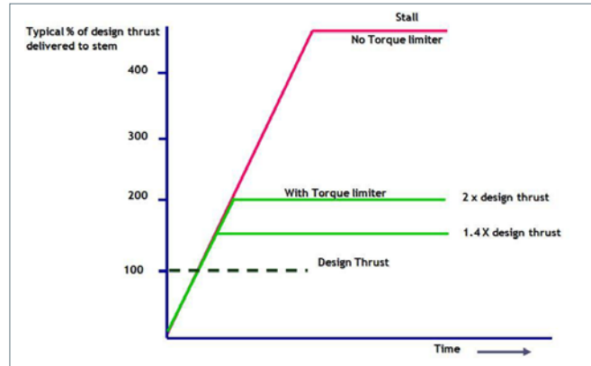
Typical Torque Limiter Performance Curve.
