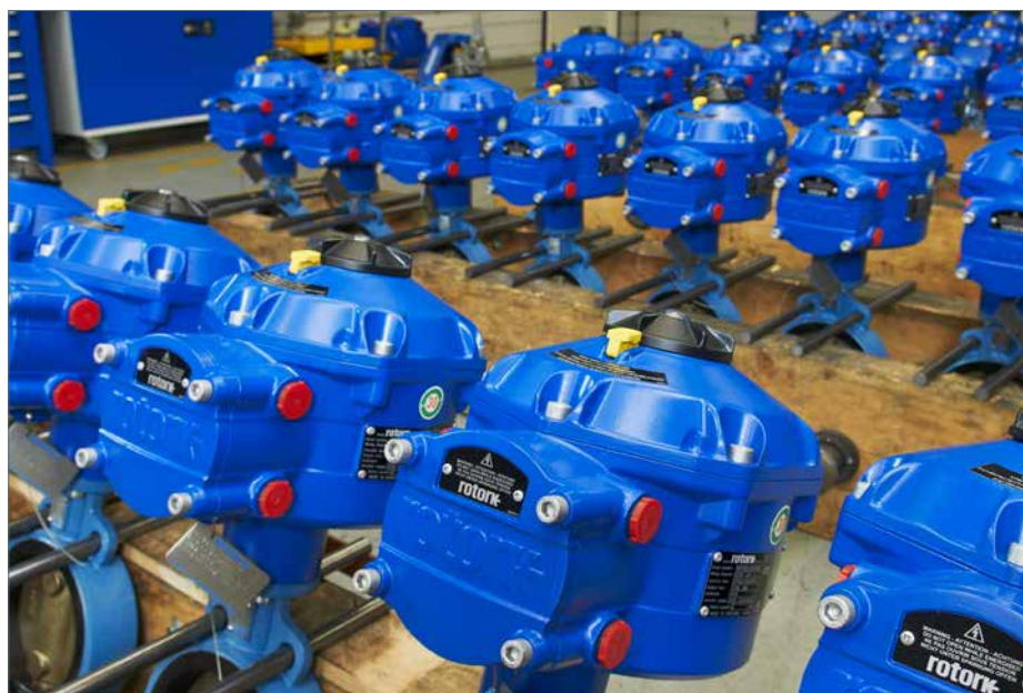
Some of the Rotork CVA actuators for the DanTysk project, fitted to butterfly valves and ready for despatch from Rotork Holland's actuation workshop facility.
