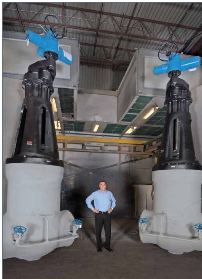
The massive size of the 36 inch high pressure parallel slide valves (16 supplied in total) is evident in this photograph.
