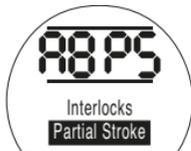
To access partial stroke test settings **PRESS THE
