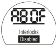
*Note: If interlocking is required in only one direction, it will be necessary to connect a link between the actuator terminals associated with the other direction. Refer to wiring diagram.*
