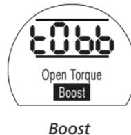
In checking mode, on pressing the
