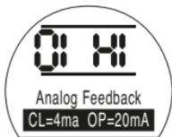
With **[HI]** Displayed, the CPT operates **Close=4mA, Open=20mA**
