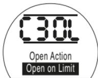
**[OL]** in the Setting Field Indicates Open on Limit.
