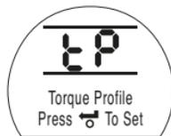
Pressing the ⏪ key stores the last measured “reference” close-open and open-close torque profiles within the datalogger.
