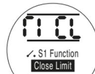
*Contact S1 Configured to Trip at Valve Closed Limit*
