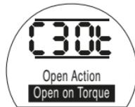
**[Ot]** in the Setting Field Indicates Open on Torque - default setting.
