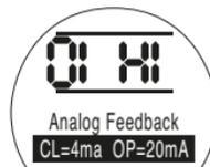
With [HI] displayed, a 20mA signal will correspond to the valve opening.
