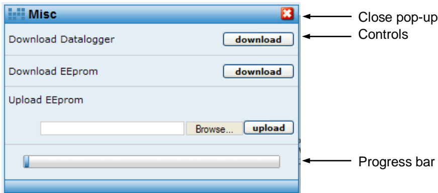
Fig 58: Wireless IQ / IQT Downloads pop-up Pop-up screen with controls to extract the Actuator Datalogger and Actuator Configuration files. It is also possible to load a configuration file to an actuator using this facility, assuming Admin login. The files that this facility creates are for viewing with the Rotork In-sight software, available on the Rotork web site.
