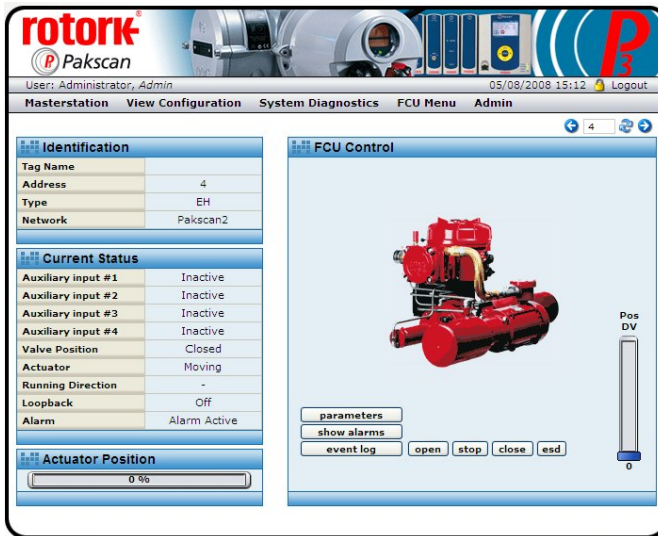
Fig 48: EH Actuator FCU Control
