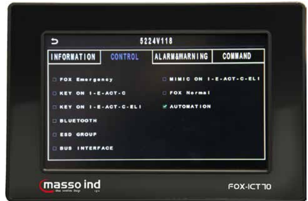
4. CONTROL PRIORITY ACTIVE on VALVE
