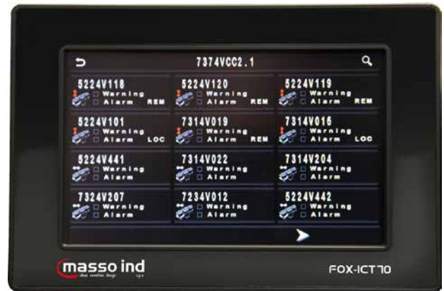
2. VALVE LIST with Feedback and Warnings/Alarms status
