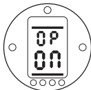
Profibus set-up screens [ON]
