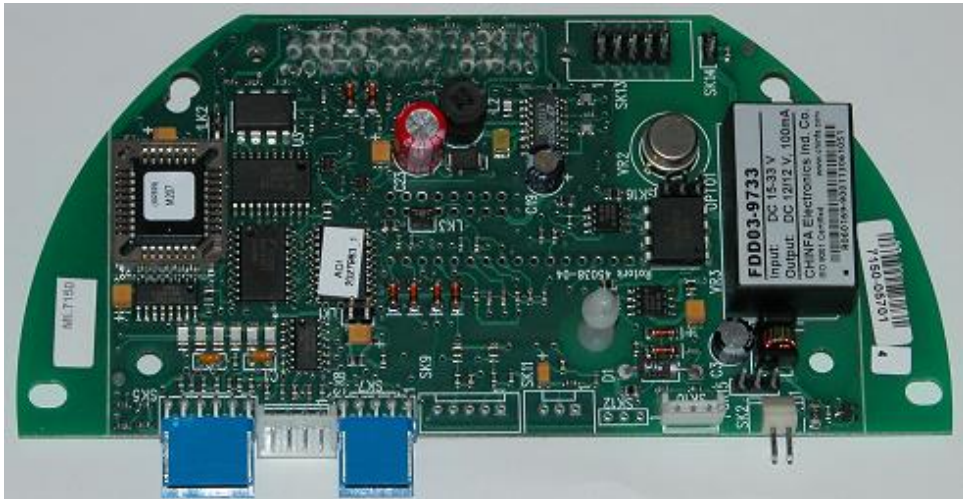
Fig 4: The Interface Card (Q and Skil/EH actuators)
