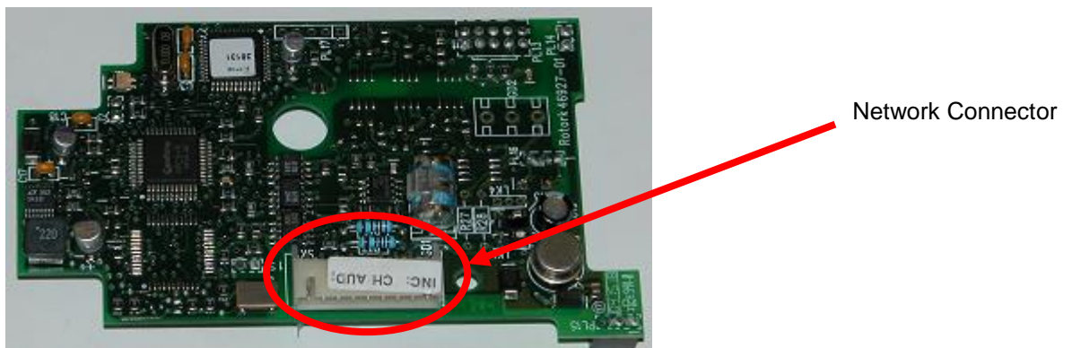
Fig 3: The Profibus single channel NIC, showing the network connector.
