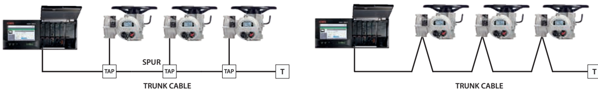
Fig 8.1.1: RS-485 Data Highway Topology – Single Channel
