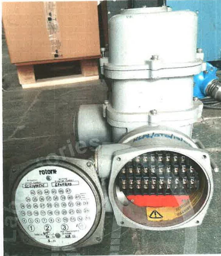
Pictute3: No ingress of powder & water observed
