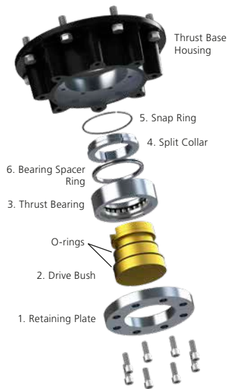
Fig. 5.1.4 F25 & F30 base assembly
