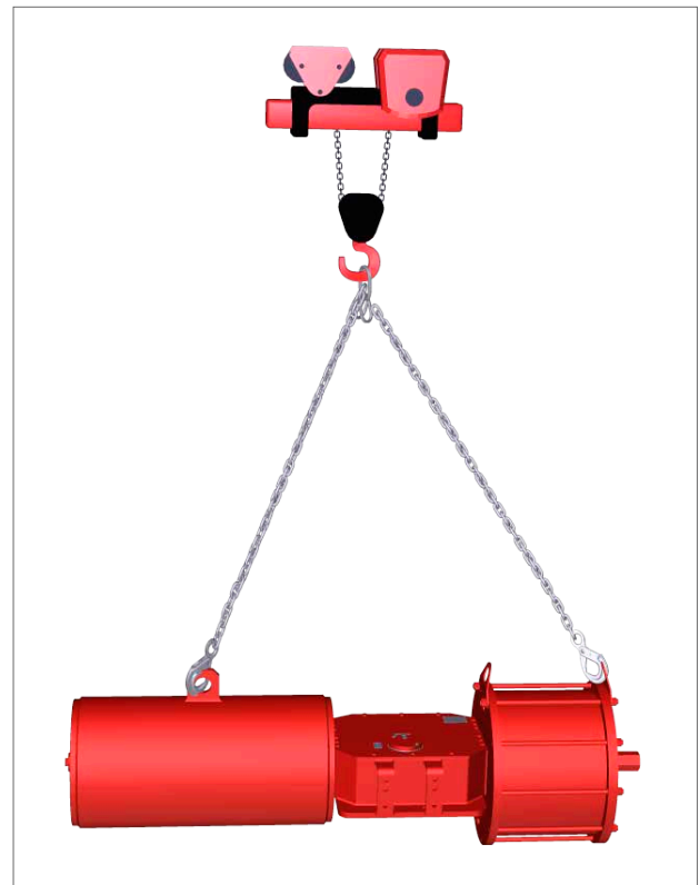
Fig 7.1 Lifting (single-acting actuator up to size 161)
