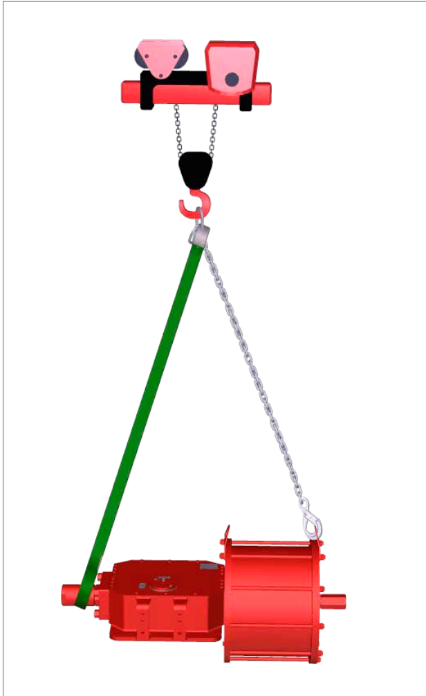
Fig 7.2 Lifting (double-acting actuator up to size 161)
