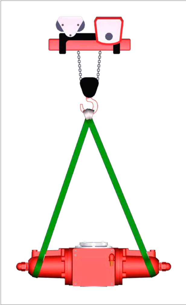
Fig 7.2 Lifting double-acting RH body sizes 015, 030, 060, 120, 240.
