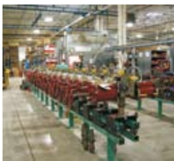
Top: Pre-compressed spring packs for 1/4 turn and linear operators in the Lucca, Italy factory.
