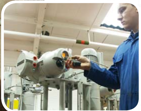
Above: Customised Rotork Skilmatic linear double-acting actuators undergoing final factory inspection, utilising "non-intrusive" programming technology.
