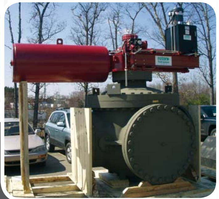
Rotork EH 200C-125/C1 actuator fitted to a GA Industries R-201-D ball valve, awaiting despatch to the Baumgartner Lift Station.
