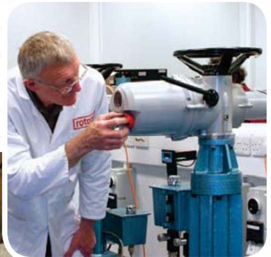
Above: A Rotork IQM intelligent electric modulating actuator in the company's R & D laboratory.
