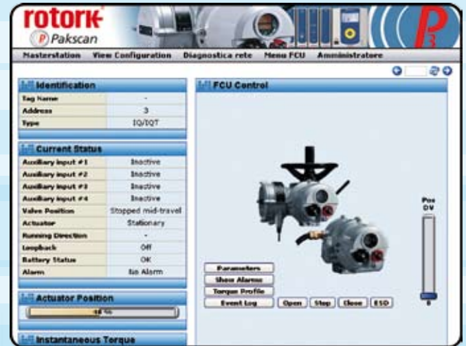
Web Browser - MOV Control & Monitoring
