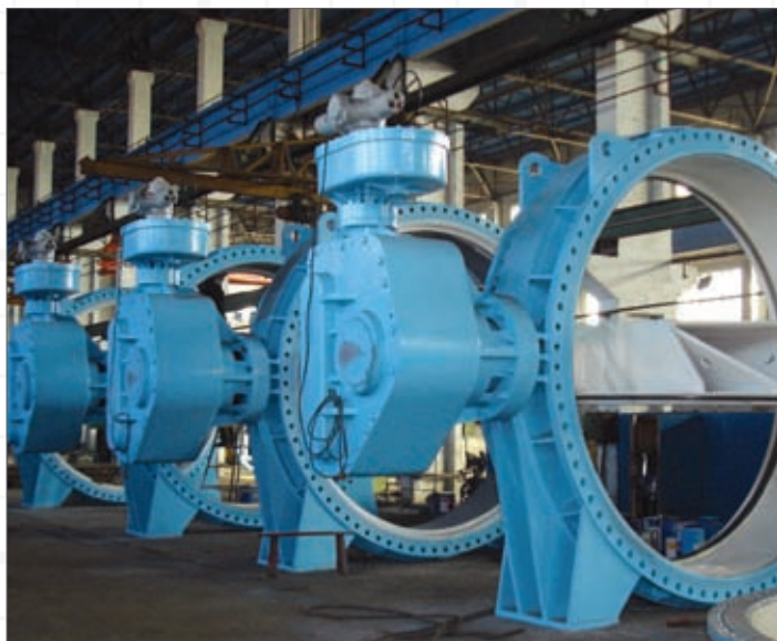
Rotork IQPro 35 actuators photographed at the Tielin Valve factory in China, fitted to 2400mm diameter pipeline butterfly valves for the Dahuofang Water Supply Project
