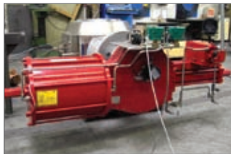
GP range pneumatic actuator with manual hydraulic override
