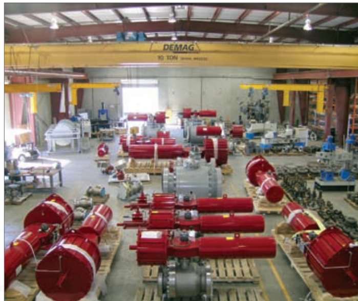
Some of the valves and actuators for the Meeker Gas Plant at the DHV Industries factory
