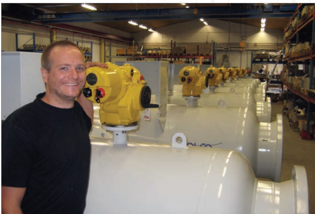
Bjorn Nilsson is pictured with some of the IQT actuated Alfa Laval water filters
