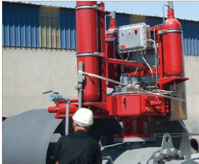
Work in progress on a Rotork GO Range actuator and valve package en-route to Kurdistan.
