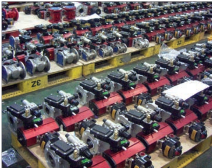
Remote Control RC200 pneumatic actuators in the Rotork Korea workshop.
