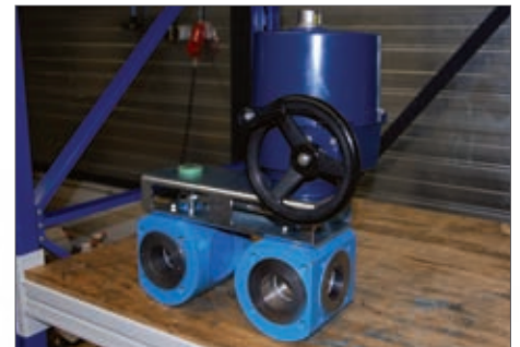
ROM actuator with customised Valvekits linkage.
