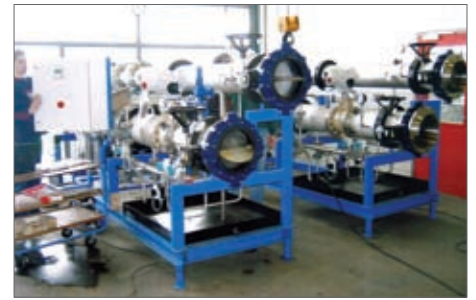
IQTM actuated valve modules for the district cooling plant.
