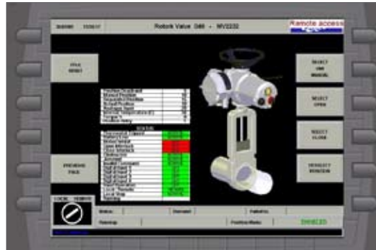
One of the Rotork actuator diagnostic touch screen HMI displays on the site's SCADA system.
