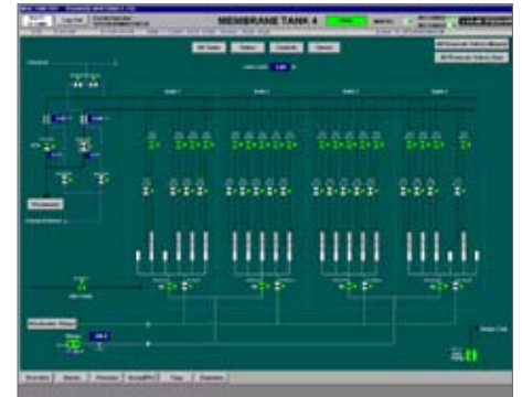
SCADA mimic screen diagram showing actuator status on one of the membrane bioreactors.
