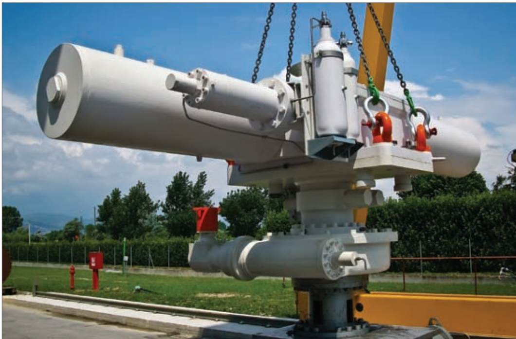
The completed actuator and gearbox assembly, with its ROV connector.
