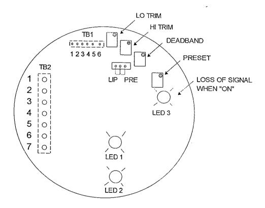
NOTES: With increasing command signal, LED 2 should be "ON"
