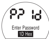
The Actuator Function Settings can be protected by the Use of a Password
