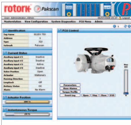
Fig. 18. Web browser - MOV control & monitoring
