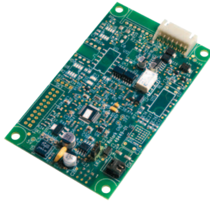
Fig. 3. An example FCU printed circuit board which are mounted within the main actuator housings
