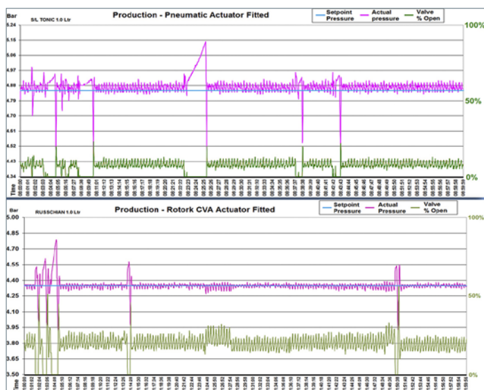
These two graphs show the improved positional accuracy of the CVA actuator in comparison with the pneumatic actuator in the production mode.
