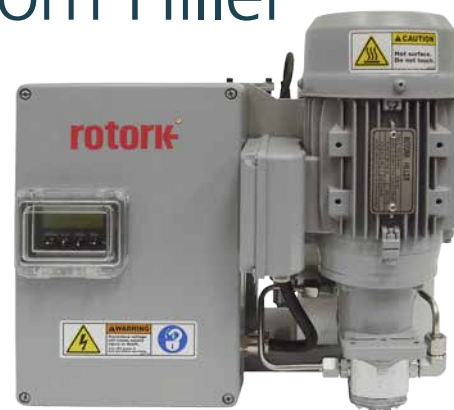
The custom-built Rotork-Hiller actuator designed for the electro-hydraulic operation of a three-way globe bypass valve within a reactor chemical water clean-up system. Restricting the overall dimensions was a critical part of the design specification, ruling out any possibility of using a standard product.
