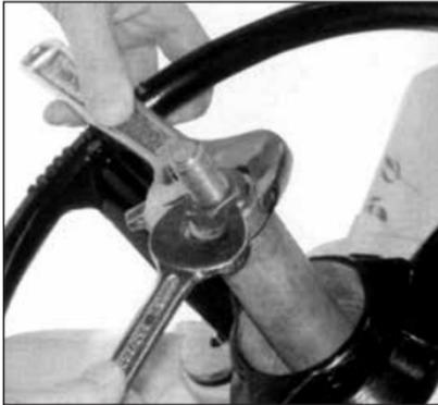
*Fig. 5.6 Down Stop two Spanners*
