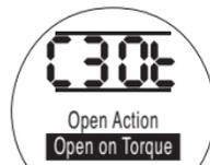
**[Ot]** in the Setting Field Indicates Open on Torque.
