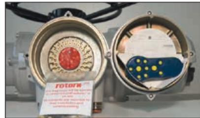
Fig. 6.2 - Actuator containing Rotork Setting Tool *Pro*.
