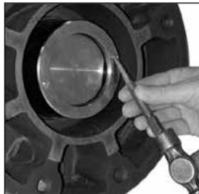
Fig. 4.6 Removal of Retainer
