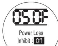
The protection may be enabled by using the + or – key to select **[ON]**
