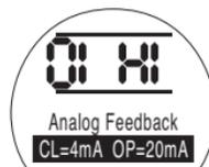
With [HI] displayed, a 20mA signal will correspond to the valve opening.
