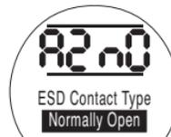
*Actuator Responds to a Normally Open ESD Contact (Signal Applied)*
