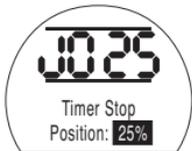
*Timer Set to Stop Pulsing when Opening Valve Reaches 25% Open*
