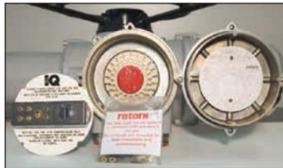
Fig. 6.1 - Actuator containing Rotork Setting Tool.
