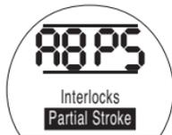
To access partial stroke test settings **PRESS THE
