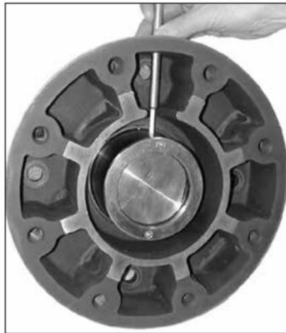
*Fig. 4.12 Tightening Retainer Set Screw*
