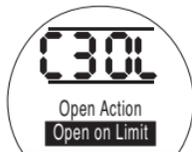
**[OL]** in the Setting Field Indicates Open on Limit - default setting.
