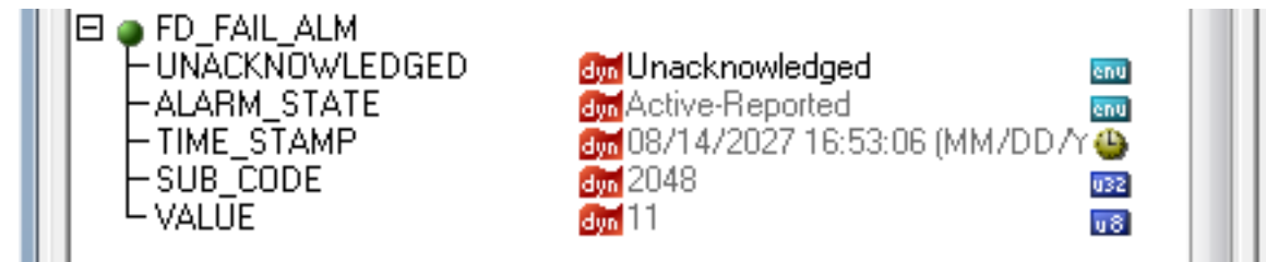
Fig E.9: Alarm state reported.
