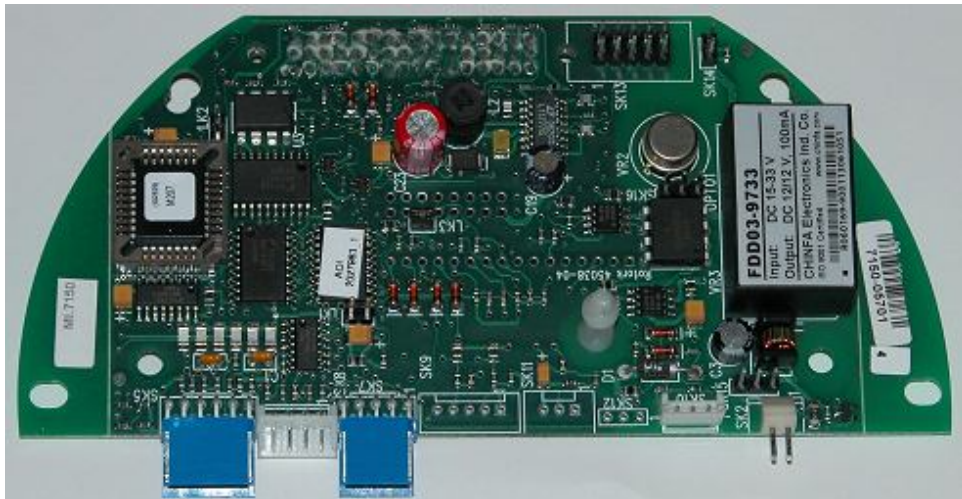
Fig 5: The Interface Card (SI Pro and EH Pro actuators, Q is similar, see Section 3.2)
