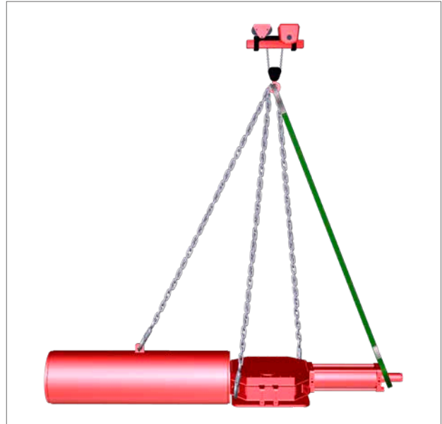
Fig 7.3 Lifting (single-acting actuator size 200 - 350)
