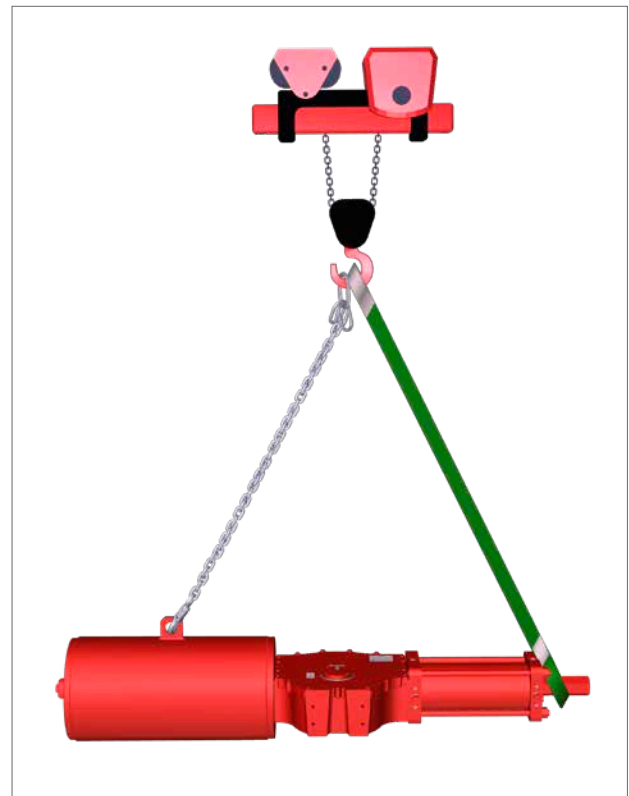
Fig 7.1 Lifting (single-acting actuator up to size 161)
