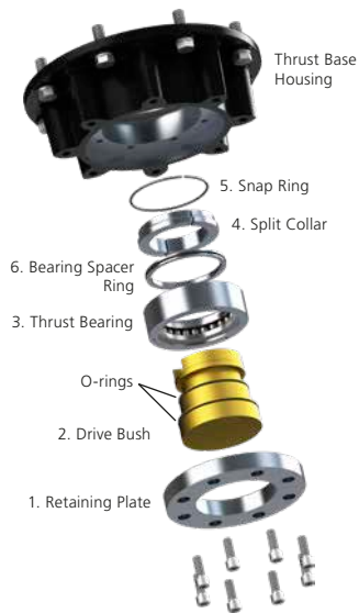
Fig. 5.1.4 F25 & F30 base assembly
