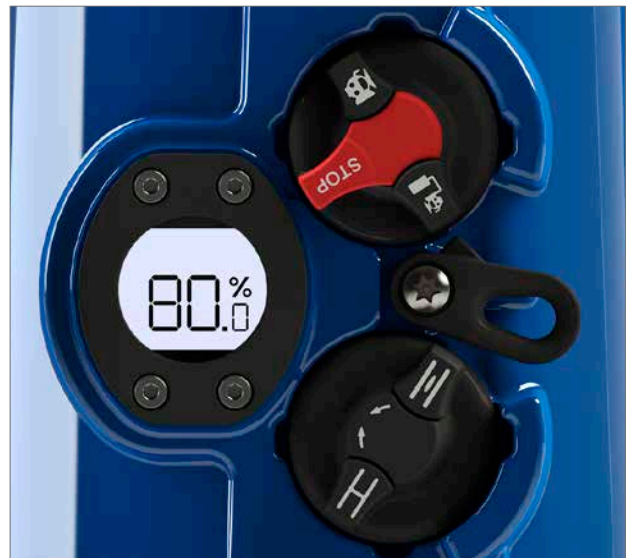
Fig 9.2 Actuator set to 'STOP' position
