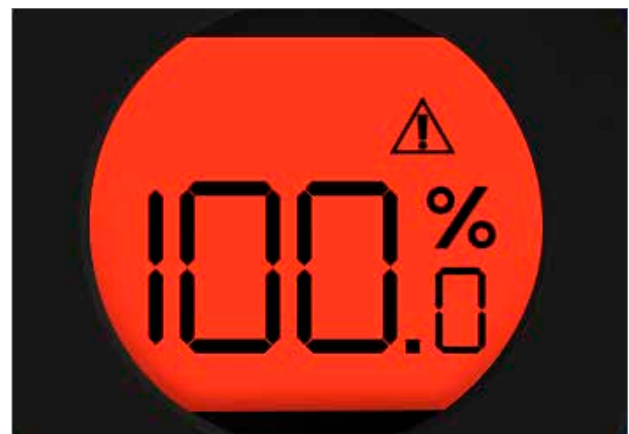
Fig 5.7 Actuator flashes Red and White alternatively when power failure occurs
