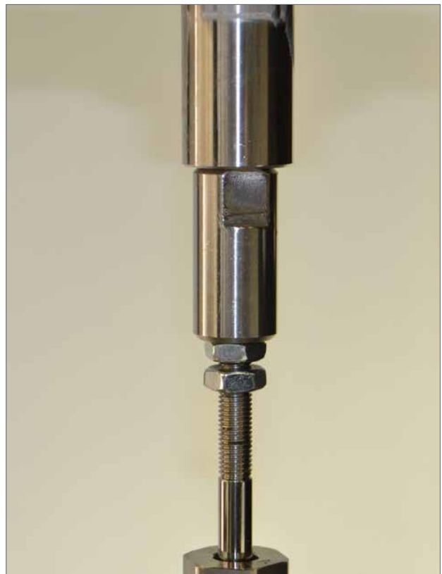
Fig 6.7 Connection of valve shaft and actuator shaft
