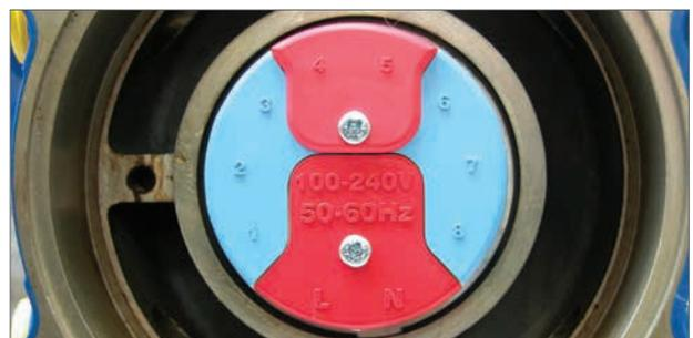
Fig 7.16 IS Terminal Block
