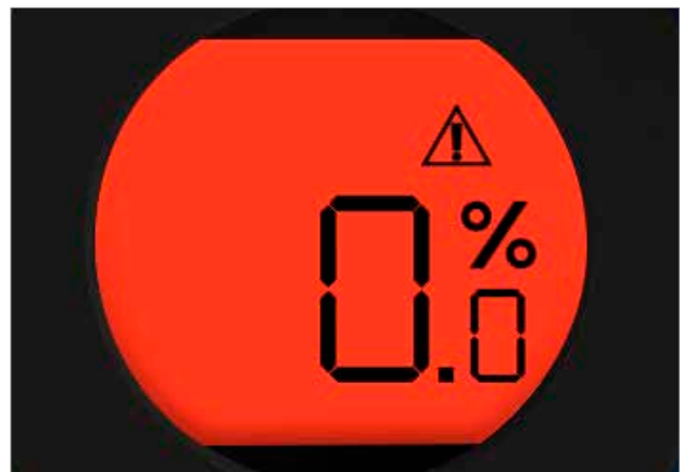
Fig 9.3 Actuator display flashes Red and White when RPP is active during power failure.
