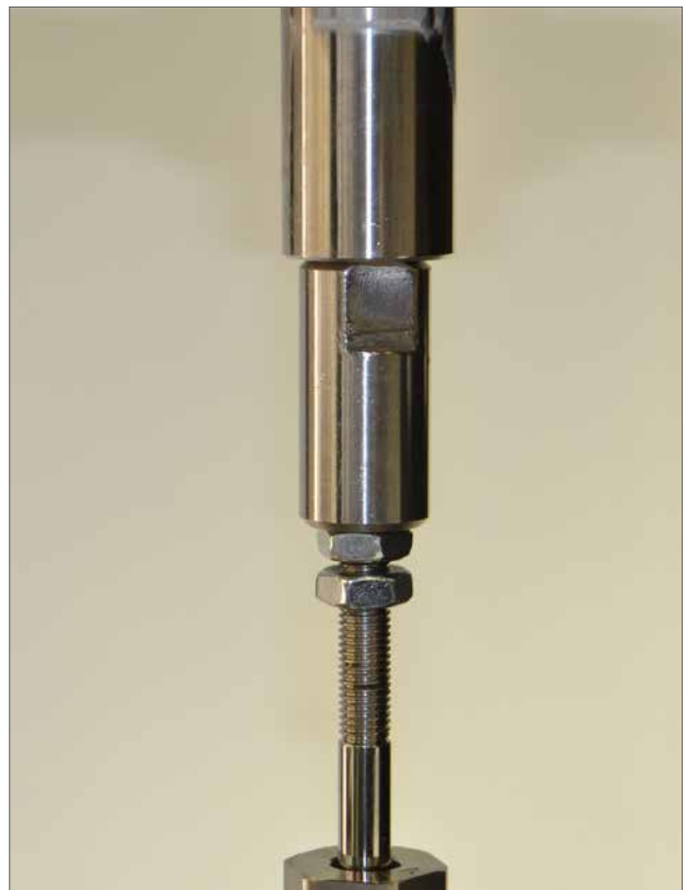
Fig 6.7 Connection of valve shaft and actuator shaft
