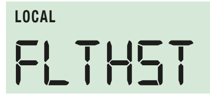
Fig 9.1 Fault history menu
