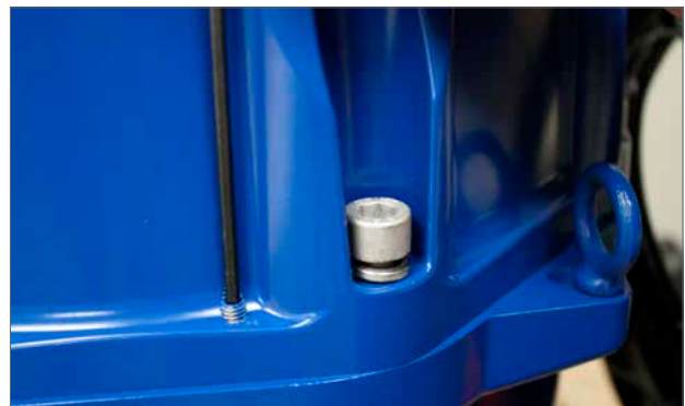
Fig 6.12 Set screw location
