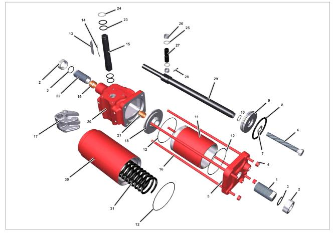
Fig 17.3 Single-Acting Actuator (size 055-065) with adapter plate
