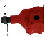
R. To increase angular stroke, rotate the stop bolt (1) anti-clockwise
