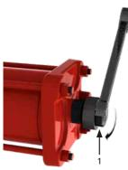
5. To decrease angular stroke, rotate the stop bolt (1) clockwise
