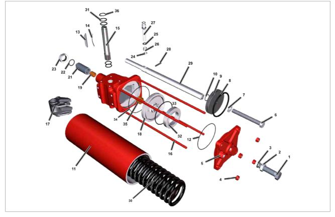
Fig 17.1 Single-Acting Actuator (size 035-045) with adapter disk
