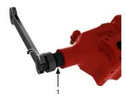
S. To decrease angular stroke, rotate the stop bolt (1) clockwise
