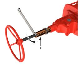
E. To decrease angular stroke, rotate the stop bolt (1) clockwise
