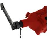
5. To decrease angular stroke, rotate the stop bolt (8) clockwise.
