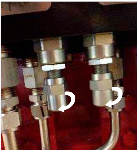
Fig 12.6 Flow regulator cap removal
