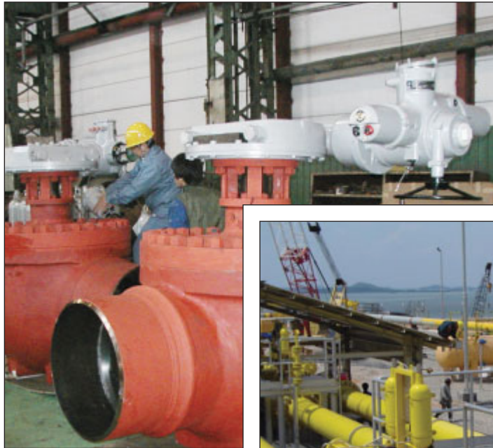
Above: IQ intelligent electric actuators fitted to Hatanaka ball valves.
