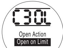
[OL] in the Setting Field Indicating Open on Limit (default).
