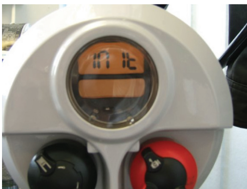
Commissioning mode initialised
