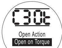
[Ot] in the Setting Field Indicating Open on Torque.
