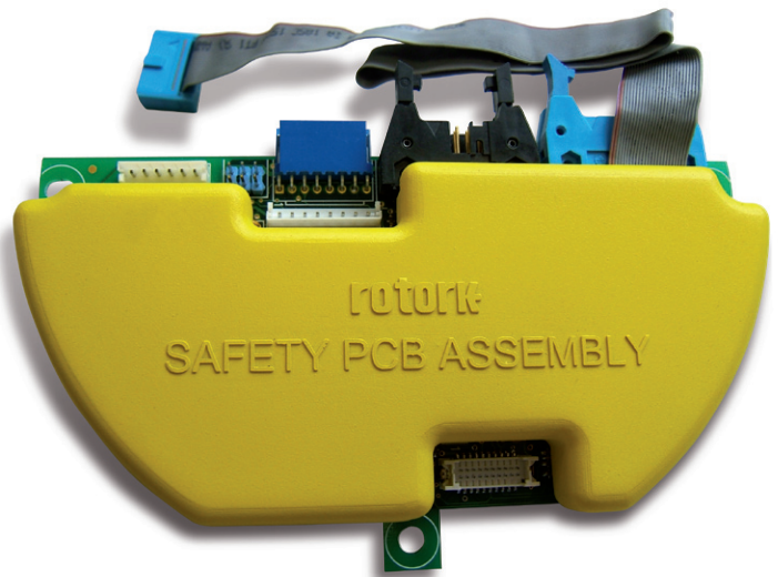
Safety Function Control Module (SFCM assembly)
