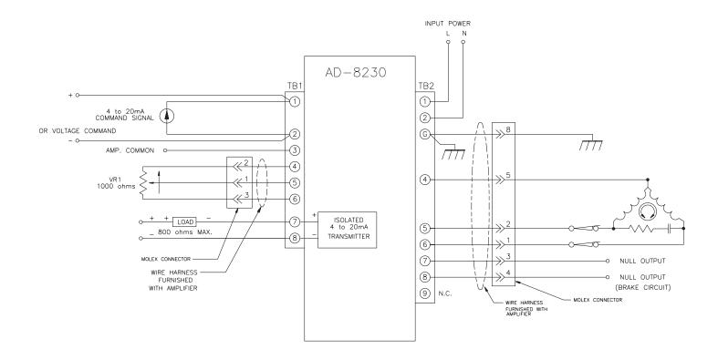
NOTE: When replacing AD-8210 or AD-8220 with this amplifier, remove and relocate field wiring as follows:
