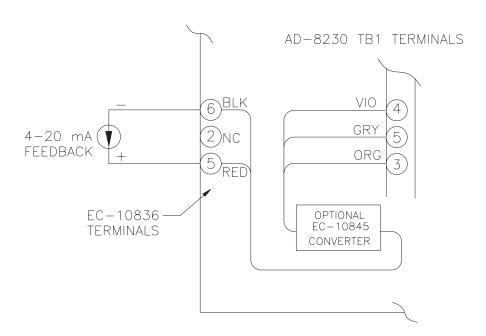
NOTE: The above diagram illustrates 4 to 20mA position feedback signal with customer supplied loop power. An optional 24 Vdc loop power supply is also available from Jordan. Refer to the wiring diagram furnished with the actuator for special calibration instructions when 4 to 20mA feedback is furnished.
