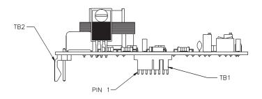
NOTE: When retrofitting the AD-8130 to replace models AD-8110 or AD-8120, note that the actuator mating connector for TB1 is a 6 pin connector that should engage pins 1 through 6 only. Pins 7 and 8 are 4-20mA outputs for new installations and are not used for replacements. (Note location of pin 1 on above drawing; pins are numbered left to right.) Contact factory if your connectors are located on the component side of the board.
