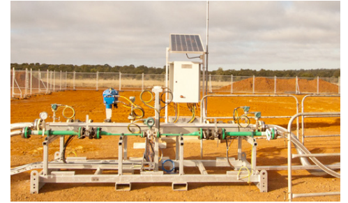
Fig 2 - In the coal mining industry, remotely sited wellhead skids designed for degassing duties are used in conjunction with control and telemetry systems to enable methane and other flammable gases to be extracted from underground coal seams prior to the commencement of mining operations.
